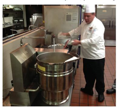
As part of this commerical foodservice research project, the chef demonstrated the advantages of a steam jacketed kettle compared with using a stock pot on a range.
